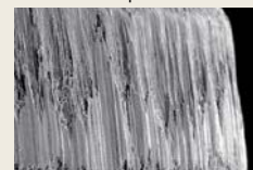
Rough, uneven wear
